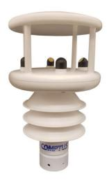
Welcome to the Comptus A70H-UWS Automatic Weather Station. The instrument does not have any moving parts, needs no maintenance, and no on-site calibration. In order to get the most out of your instrument, we recommend you read this manual carefully before installation.
